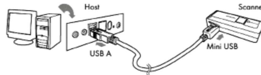
Flip the rubber cover up to expose the mini USB port on the scanner. Insert the mini USB cable into the port on the scanner and into the port on the host computer. Charge for at least 5 hours.
